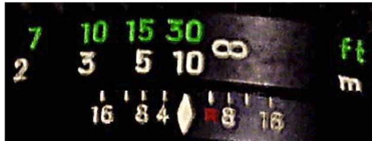
With f/8 set to infinity, the nearest distance in good focus is 5m. Consequently since 5m corresponds to half the hyperfocal distance, then at f/8 the hyperfocal distance is 10m.
